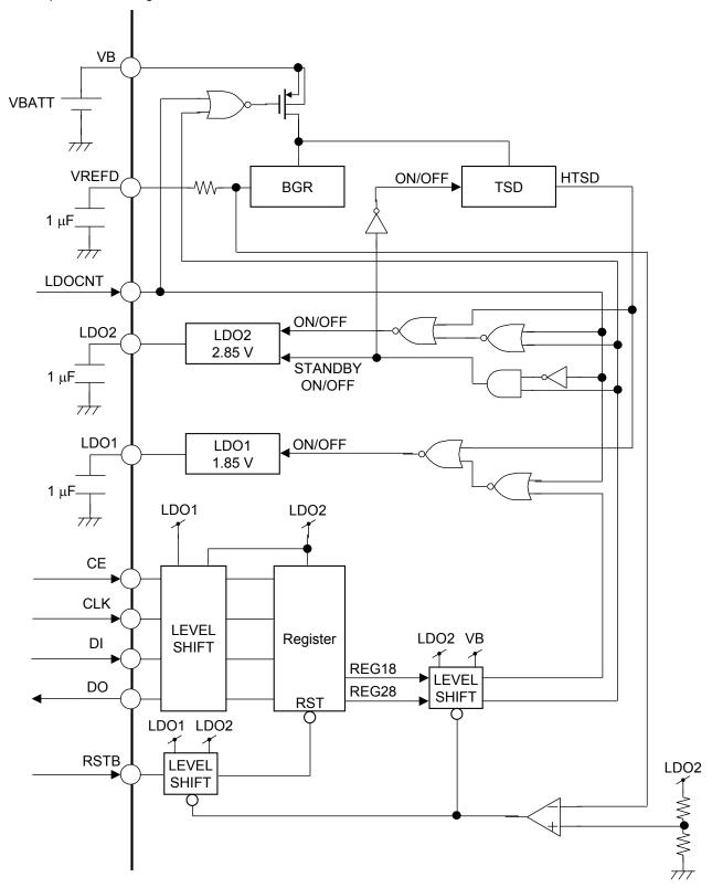
All the logic portions to which the power supply is not connected are connected to VB as power supplies.
